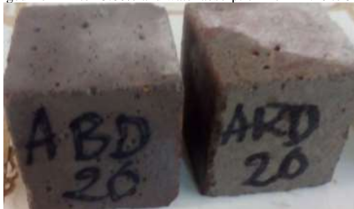
Figure 4:: Appearance of ARD and ARD clay-based mortar specimens
