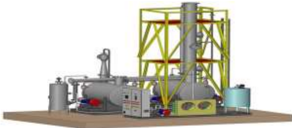
Figure 8: H 2 S Chemical Scrubber plant
