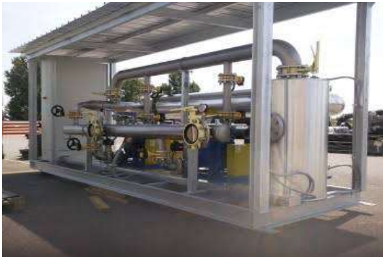
Figure 10: Dehumidifier for biogas
