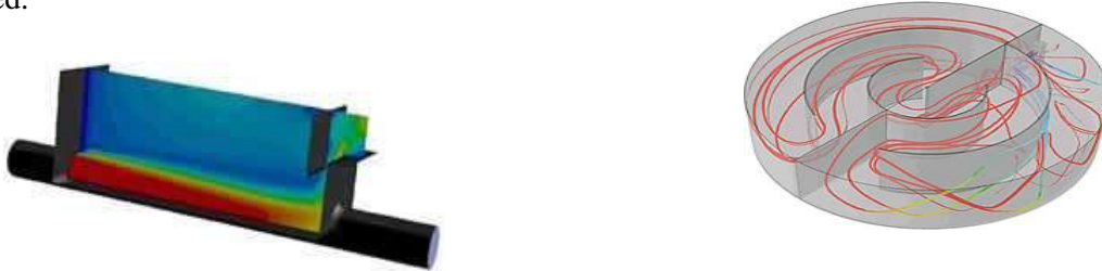
Figure 10: Contours show velocity magnitude in a symmetry plane Figure 11: Path ribbons colored by residence time in contact basin
