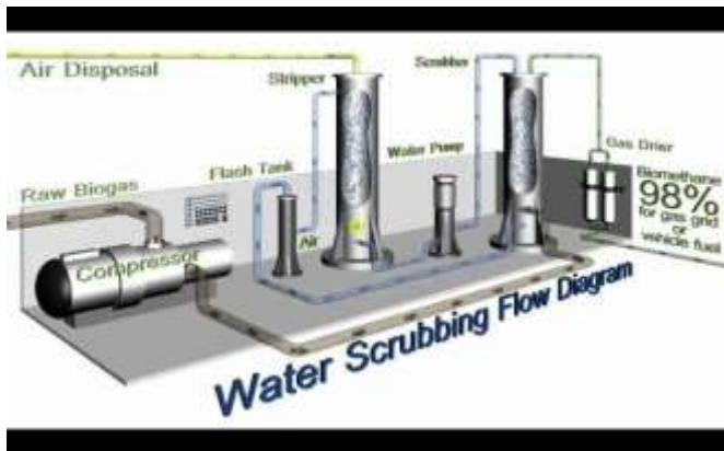
Figure 12: Water Scrubbing Flow Diagram
