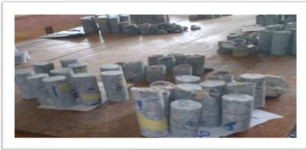
Figure 2: Prepared Cored Samples for Determination of Bulk Density
