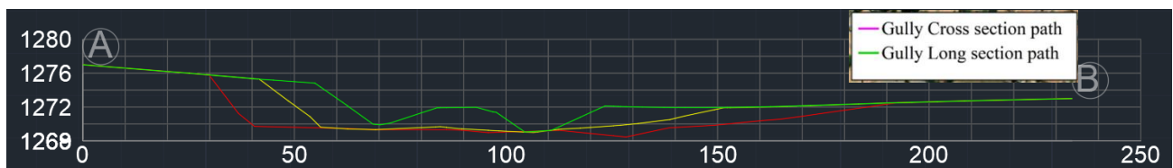
Figure 9: Gully Cross section showing profile over time in Civil 3D (units in meters).
