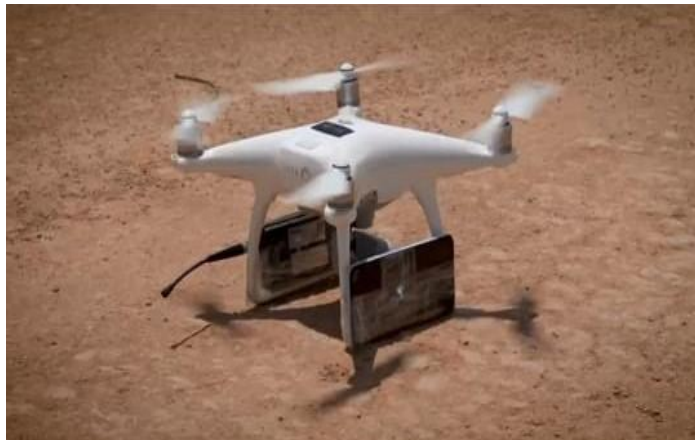
Figure 5: A converter and a mobile device onboard a drone.
