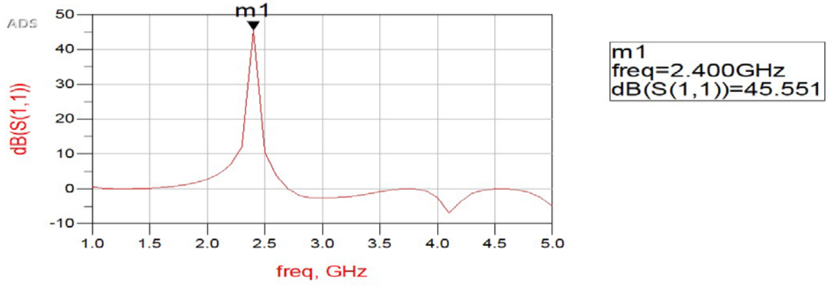
Fig. 5: |S_{11}| in (dB) versus frequency for the 2.4 GHz negative resistance oscillator
