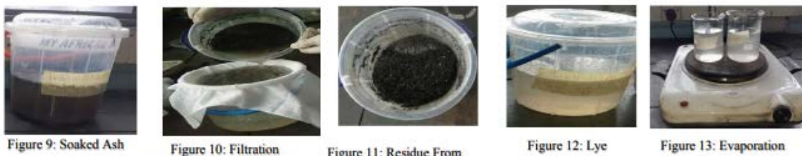
Figures 9, 10, 11, 12 and 13 Explaining the Extraction of Lye from Hardwood Sawdust and Evaporation of the Lye Extract for better Concentration.
