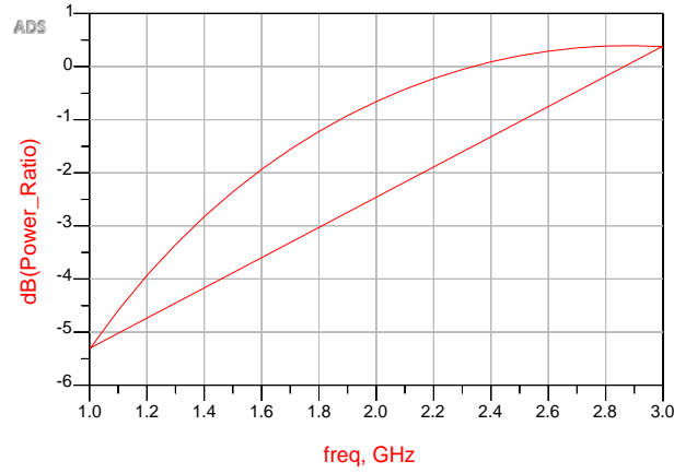
Fig. 20: Output power ratio between port 2 and 3 versus frequency of the 2.4 GHz Lang coupler
