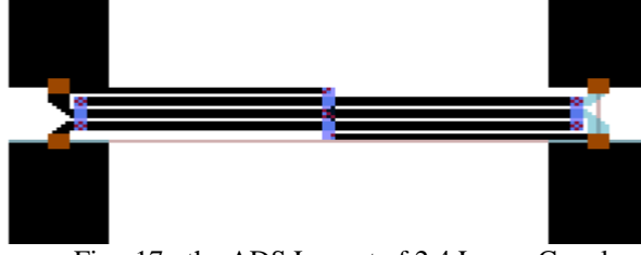
Fig. 17: the ADS Layout of 2.4 Lange Coupler.
