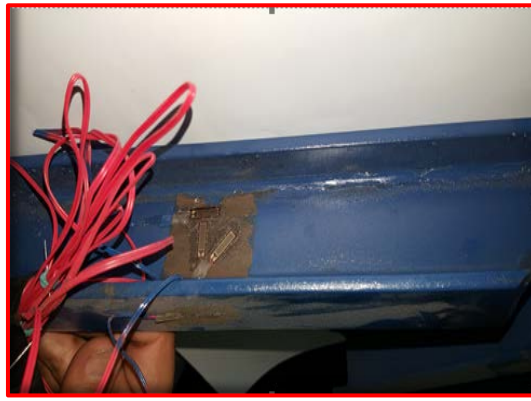
Figure (7): Electrical Strain Gauges of Steel Shear Heads.
