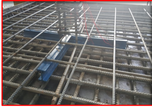
Figure (3): Specimens with Steel Shear Heads during Casting
