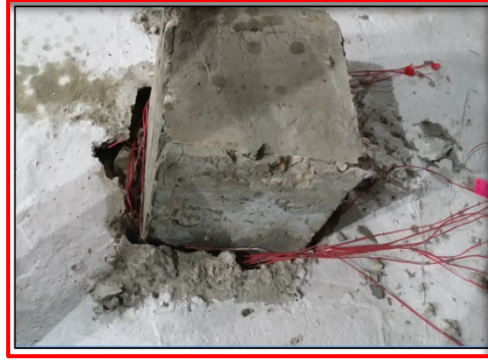
Figure (10): Crack Pattern at Compression Zone of Specimen with Shear Heads.
