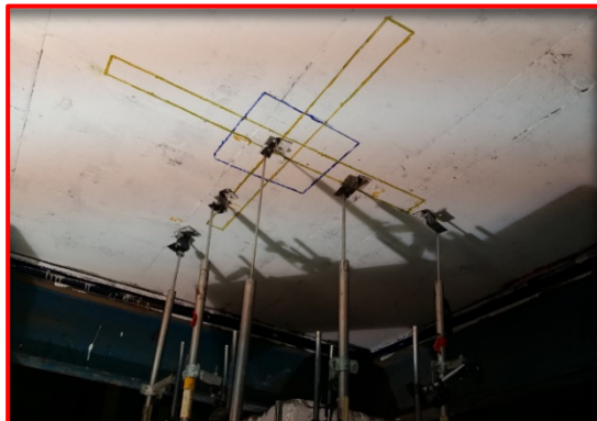
Figure (6): Arrangement of LVDTs over the Specimen.
