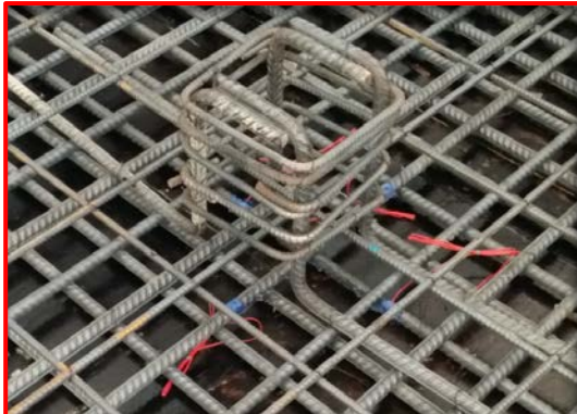
Figure (5): Locations of Steel Strain Gauges.
