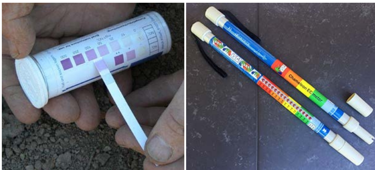
Figure 3: Nitrate strip (4a) and Chameleon EC meter (4b) used to show how much nitrate is there within a particular soil depth and electrical conductivity respectively
