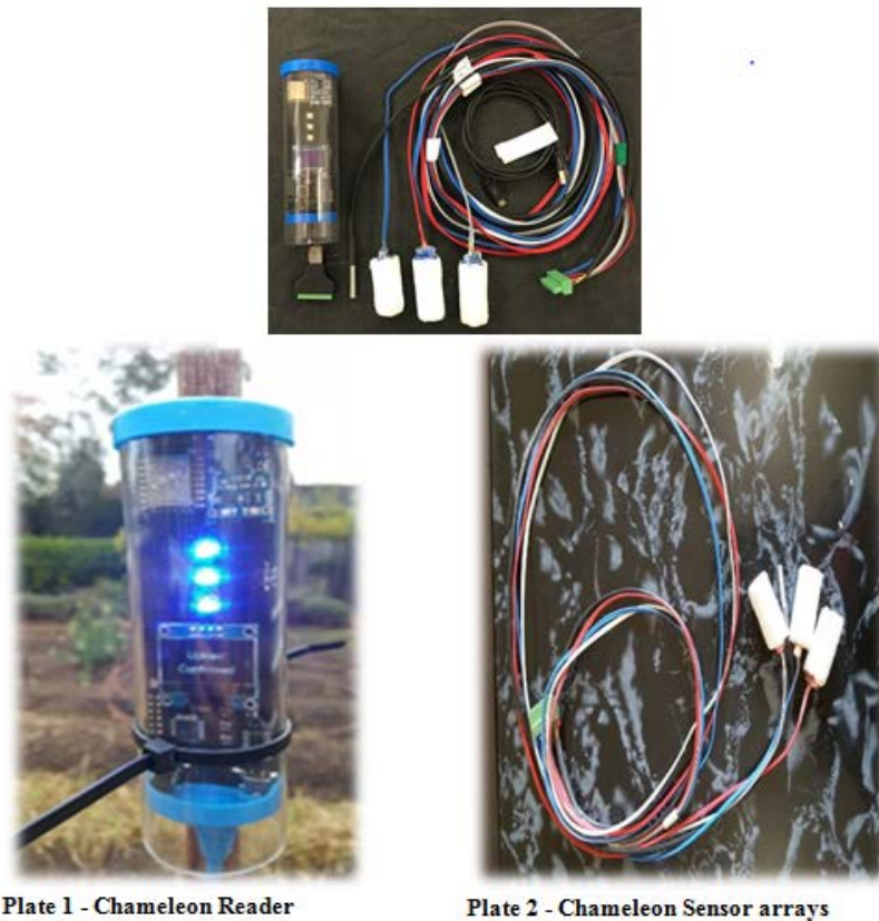
Figure 1: The wi-fi chameleon reader (plate 1) and chameleon sensor arrays set (plate 2)
