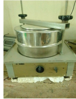
Figure A9: Sieving of crushed samples with an electric shaker (Snail shells)
