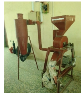
FigureA3: Hammer mill for the crushing of the periwinkle and snail shells
