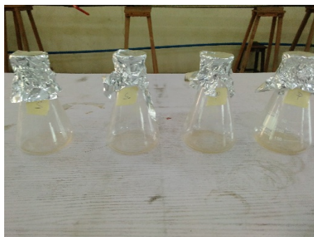
Figure A19: Diagram of diluted crushed samples (CPS & CSS) for titration
