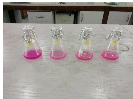
Figure A20: Diagram of end point of titrated samples (CPS & CSS)
