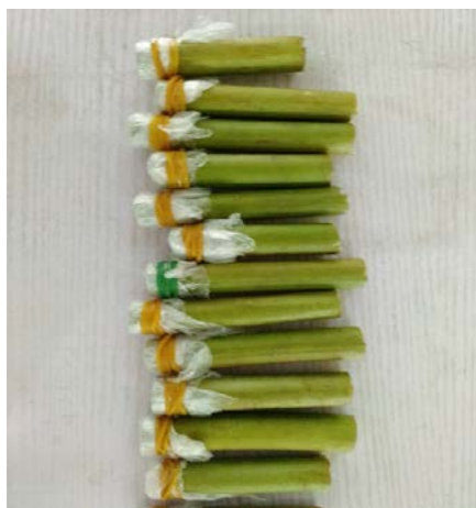
Figure A21: Diagram of prepared pawpaw straws as moulds
