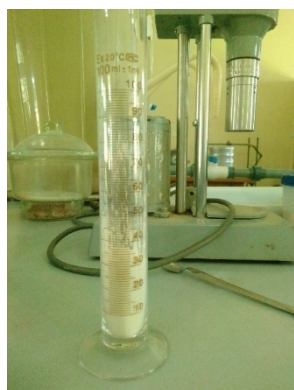
Figure A18: Sample of CSS in graduated cylinder for bulk density measurement
