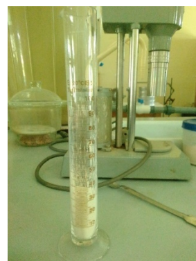
Figure A17: Sample of CPS in graduated cylinder for bulk density measurement
