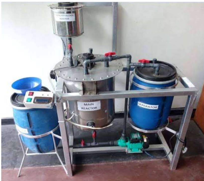
Figure 6: Compact Biodiesel Production Plant for Moringa Seed Oil.
