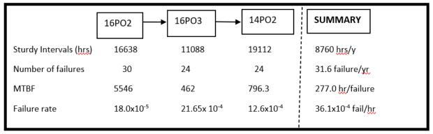
Also from the failure rates the lost time per pump is calculated and the overall lost time for the system is determined as 756.68hrs/yr. From the figure below we also see money lost from pump failure and set priorities.
