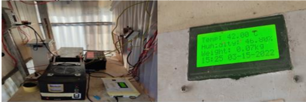
Figure 4: 2kVA Inverter, Batteries, Charger Controller and Microcontroller Data Logger
