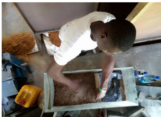
Plate 5: Preparation of Corroded Soil sample
