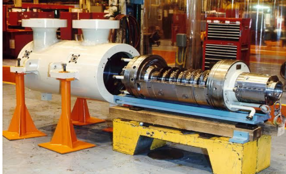
Figure 5. Centrifugal Compressor Casing Models. (Left: Removing a Bundle Using a Barrel-Style Compressor [Courtesy Solar Turbines Incorporated], Right: Compressor with a Horizontal Shaft [Courtesy Dresser-Rand Company]).
