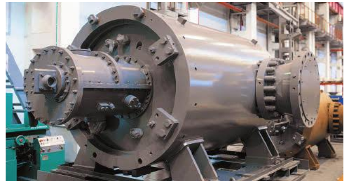
Figure 5. Centrifugal Compressor Casing Models. (Left: Removing a Bundle Using a Barrel-Style Compressor [Courtesy Solar Turbines Incorporated], Right: Compressor with a Horizontal Shaft [Courtesy Dresser-Rand Company]).
