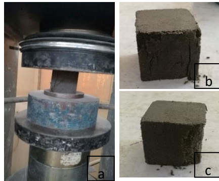
Figure 3. Compressive strength recovery: a) compressive strength machine, b) control mortar specimen, c) mortar cubes with encapsulated bacteria specimen.
