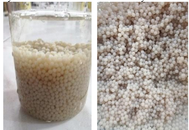
Figure 2. Encapsulated bacteria in concrete mix.
