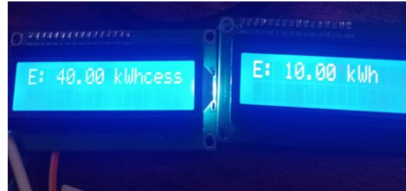
Fig 6: Updated meter status after successful transfer of 10kWh
