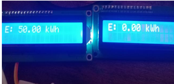
Fig 5: Meter status before sharing of electricity units
