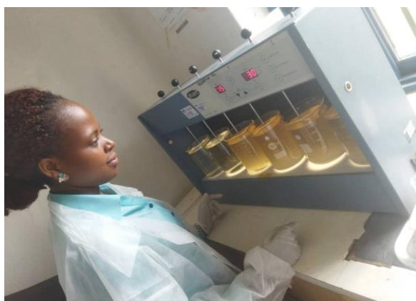
Fig. 5. Mixing raw water with coagulant
