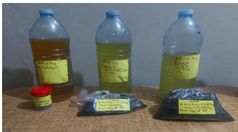
Fig. 2 shows the difference between oil formed in the absence and presence of a catalyst
