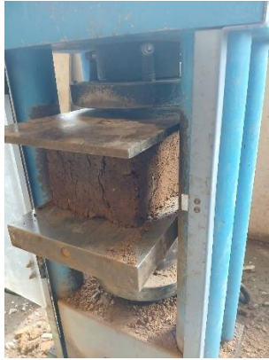
Fig. 3: Compressive strength test on the blocks at 180 days.
