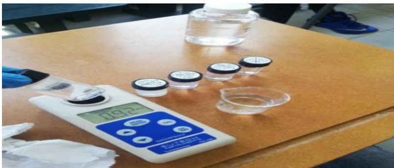
Fig. 4: 18 Test kit – Colilert method (Source: University of Johannesburg, Water and Health Research Centre (2019))
