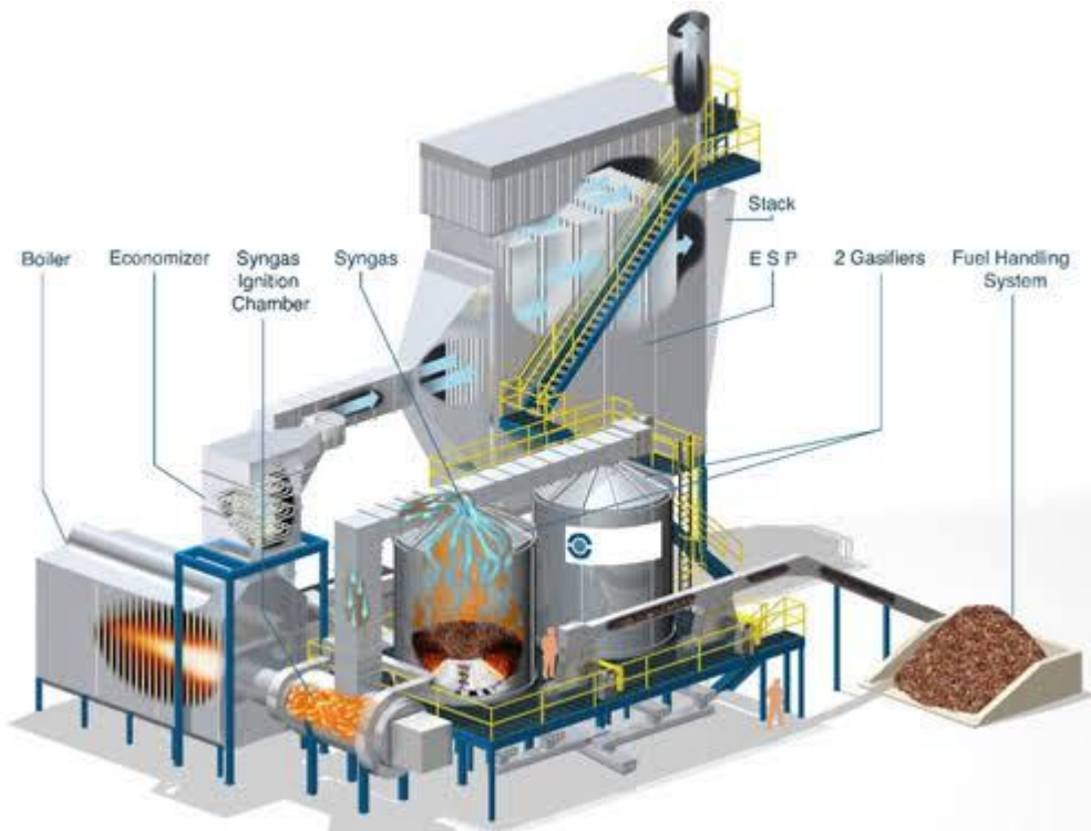
Fig 5: The Biomass Gasification power plant System
