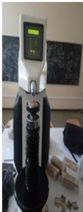
Fig. 7. Experimental setup of hardness test and the general characteristics of hardness testing methods and calculating hardness (Digital Hardness tester Machine, made in China).
