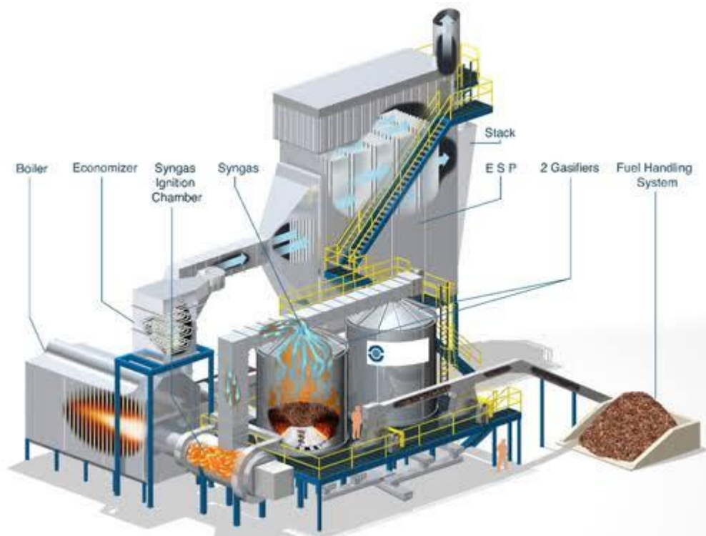
Fig 5: The Biomass Gasification power plant System
