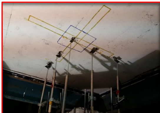
Figure (6): Arrangement of LVDTs over the Specimen.
