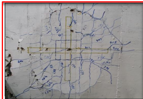
Figure (9): Crack pattern at Tension Zone of Specimen with Shear Heads.
