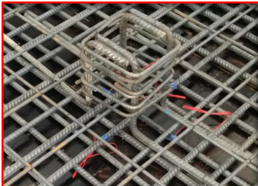
Figure (5): Locations of Steel Strain Gauges.
