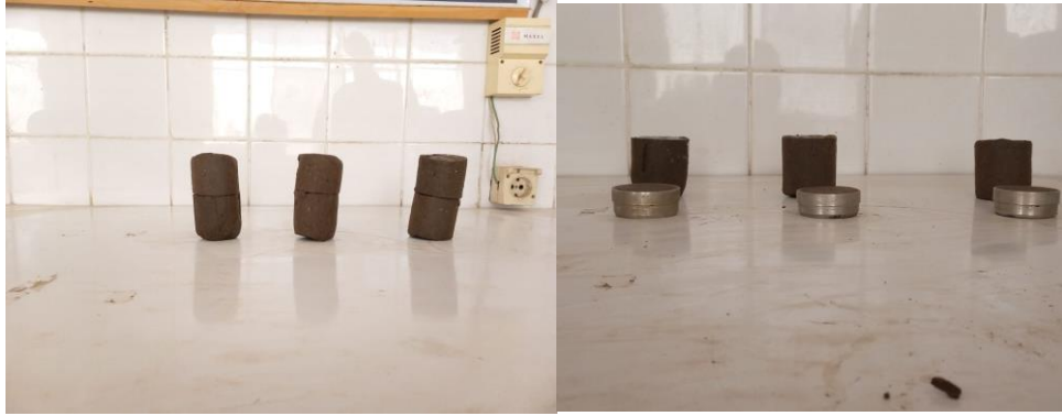
Fig. 2: Preparation of soil samples for consolidation testing.
