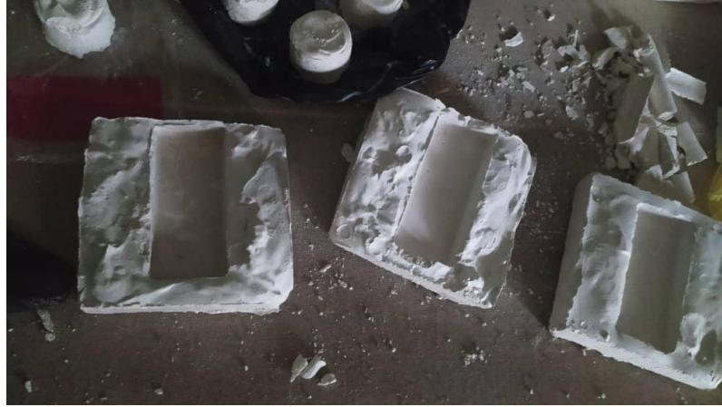
Fig. 1: Moulds for Flexural Strength Samples
