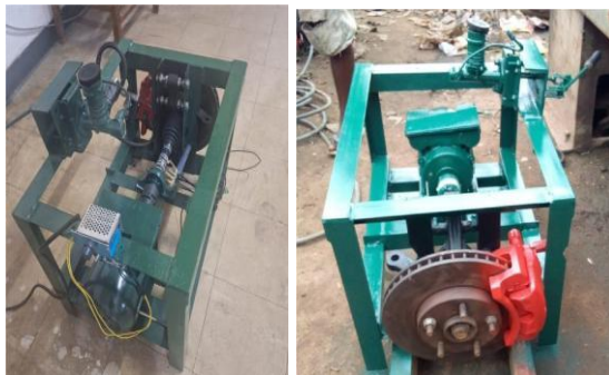
Fig. 8: Full assembly of the brake fluid tester dynamometer
